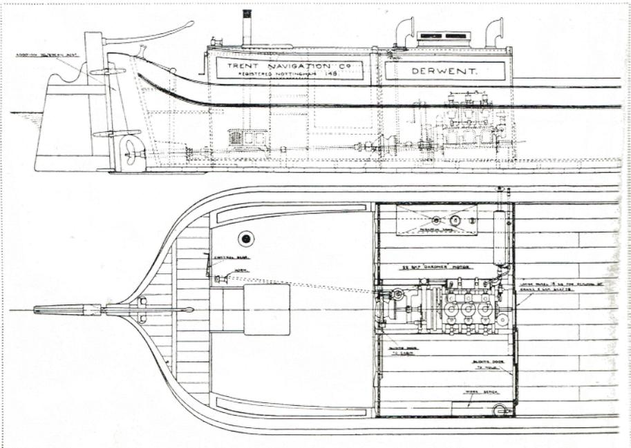
*Plans of machinery space and cabin of motor barge "Derwent."*
