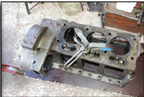
A notable difference between an L2 and the LS upper crankcase that the timing cover is integral on the LS
