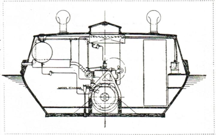
*Cross section through engine-room.*
